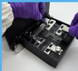
Large PDMS membrane stretch
