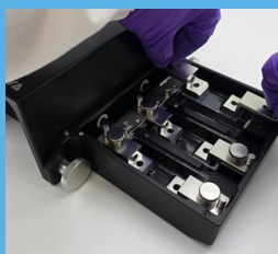
Small PDMS membrane stretch
